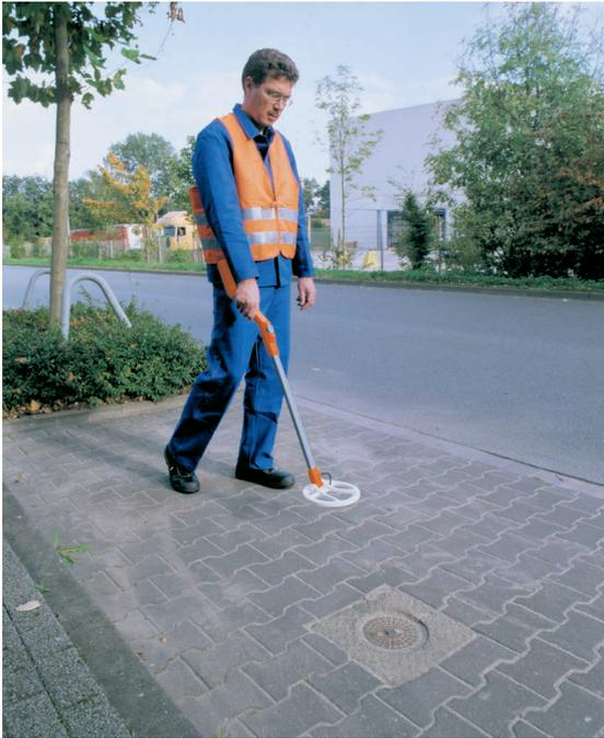
The locator M 130 detects deeply and is hardly effected by metal pieces at the surface, humidity and temperature variances. The one-button-operation simplifies the handling of the instrument, continuous re-adjustment is not necessary. The special electronics reduces false signals caused by objects such as bottle-lids, beverage cans or other small parts of metal.
